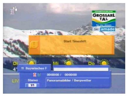
The red "T" in the info bar indicates time-shift recording. You see a freeze-frame image while the recording is running in the background. For a short time "R" flashes at the top left of the TV screen and the red standby LED on the front panel of the receiver flashes.
